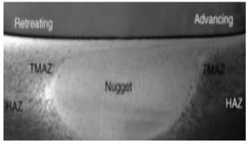
**Fig 4**. A macrograph showing various microstructural zones in FSP 7075Al-T651 (standard threaded pin, 400 rpm and 51 mm/min). [1] **3.2 Nugget**
