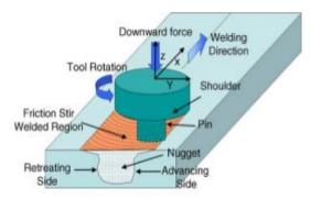
Fig.1 Friction stir welding Table 1: Benefits of Friction Stir Welding[1]
